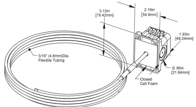
Fig. 1: Duct Averaging Transmitter with BAPI-Box Crossover Enclosure
