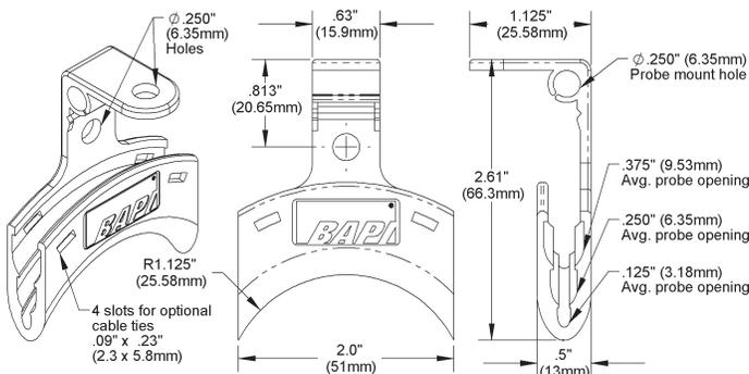
**Fig 6:** Flexible Probe Bracket (BA/FPB)
