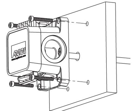
**Fig. 4:** BAPI-Box Crossover Mounting to the Duct
