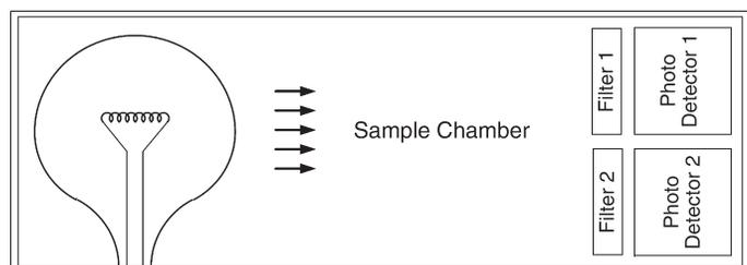
**Figure 2:** Dual Channel CO<sub>2</sub> Sensor
