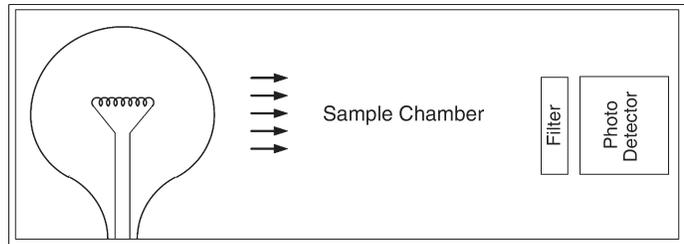
**Figure 1:** Single Channel CO<sub>2</sub> Sensor
